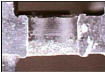
Photo 3: Trigger port: 1/2 clean; 1/6 ?; 1/3 buildup
